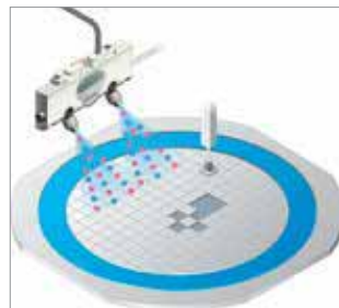
Removing charge during pickup from dicing type
