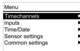
Menu navigation on the touch-surface is performed by pressing the buttons "up" (A), "down" (C), "left" (D), "right" (B) or the power button. Choose the desired parameter and press "right" (B) to open up the submenu. The menu will default after 30 seconds if no button is pressed. To exit the menu select the header line and press "left" (D).
