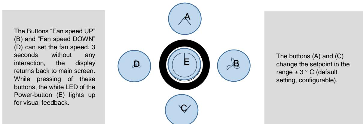
With power-button (E), the device can be set in standby mode by pressing the button (if keycard-switch function is NOT used). If the button is used as a occupancy button, the button must be pressed for at least 3s, in all other cases, a short actuation is sufficient. In standby mode, the display and all outputs are switched off (controller deactivated). The frost and heat protection monitoring remains active.
