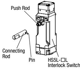
3. Pull the connecting rod from the hole in the mounting frame, and turn the button operating pin to the horizontal position.
