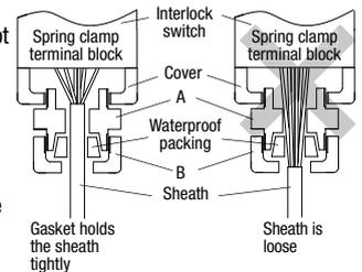
Make sure that the entire bore surface of the gasket is in contact with the sheath.
