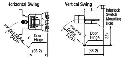
When the center of the hinged door is used as the reference for the actuator mounting surface:
