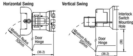
When the center of the hinged door is used as the reference for the actuator mounting surface:
