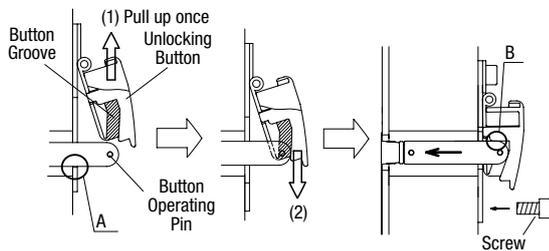
5. After fastening the screws, check if locking and unlocking operations can be performed.
