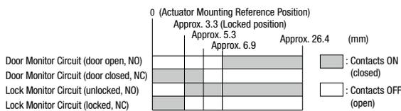
• The operation characteristics shown in the chart above are for HS9Z-A51. For other actuators, add 1.3mm.
