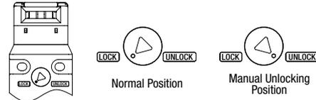
When locking or unlocking the interlock switch manually, turn the key fully using the manual unlock key supplied with the interlock switch as shown above. Using the interlock switch with the key not fully turned (less than 90°) may cause damage to the interlock switch or operation failures (when manually unlocked, the interlock switch will keep the main circuit disconnected and the door unlocked).
