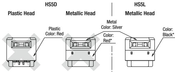
\* The metal head can be distinguished easily by the color of the plastic.
