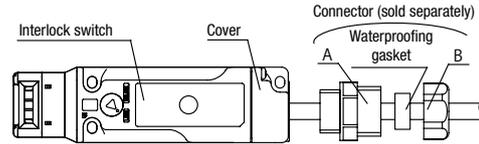
\* To remove the wiring, turn the power off and then unwire in the order of B → cover (→waterproof gasket → A).
