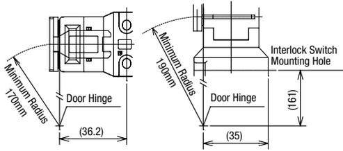
When the center of the hinged door is used as the reference for the actuator mounting surface:
