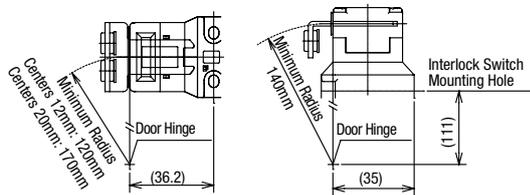
When the center of the hinged door is used as the reference for the actuator mounting surface:
