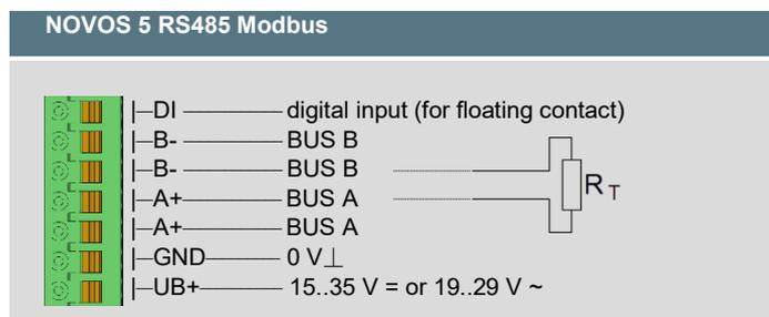
Don't forget the BUS termination (120 Ω) at the last device of the line!
