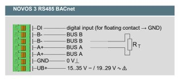
With alternating voltage, the correct polarity must be ensured!
