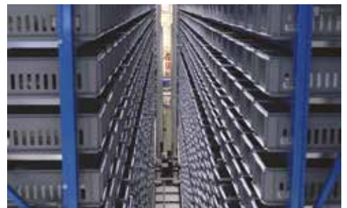
Rail dependent storage and retrieval equipment
