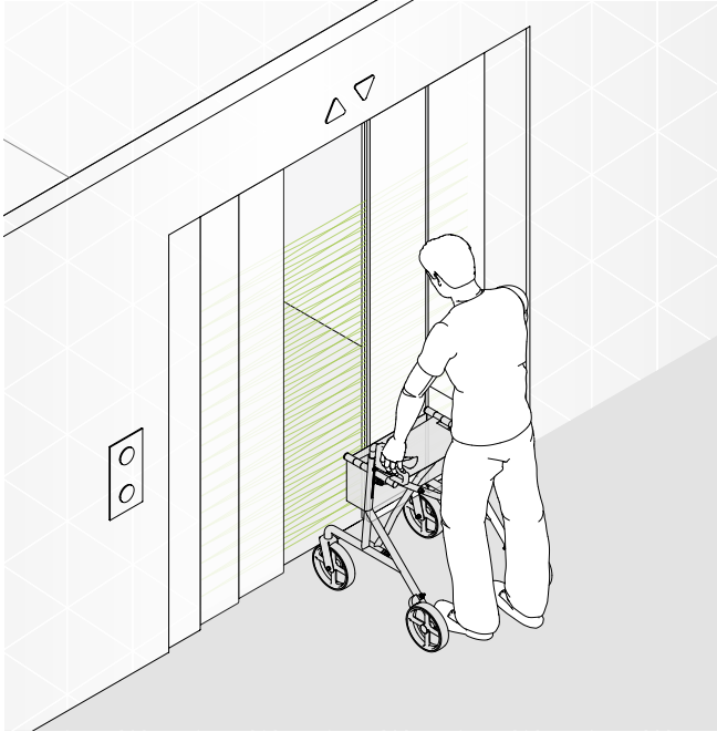
CEDES 2D light curtain technology offers reliable door monitoring.
